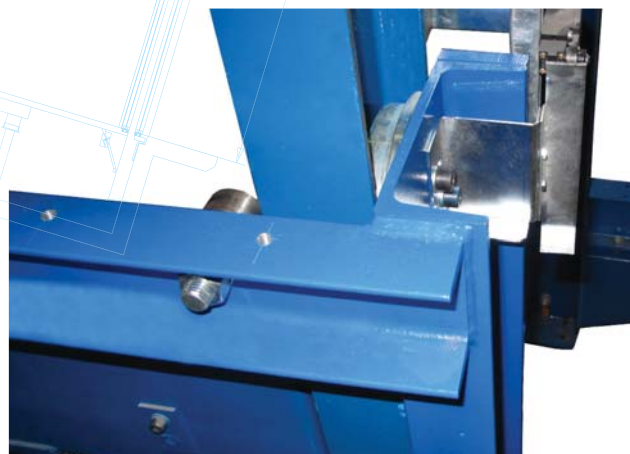
Figure 6. Lateral Guiding, 4 bearings per frame.
