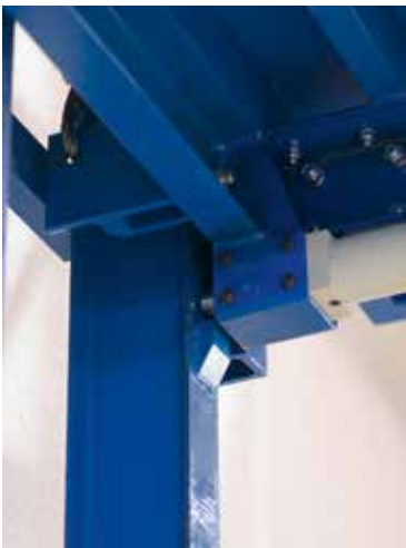
Details of the anti-creep latch
